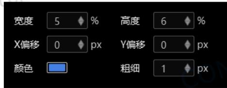
4. Set the parameters, such as thickness, position, and color, and the cross line will change accordingly in real time.
